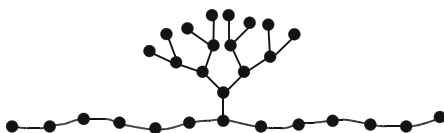
Fig. 21 Polymer chain bearing a dendritic wedge in its middle
